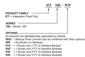
\*ICT100 includes integration client software, one high speed smart router and one high speed (TP-1250) LON interface module to connect existing wiring from legacy MacroServers. If different configurations are desired, select the appropriate options. Use the following table for ordering guidance.
