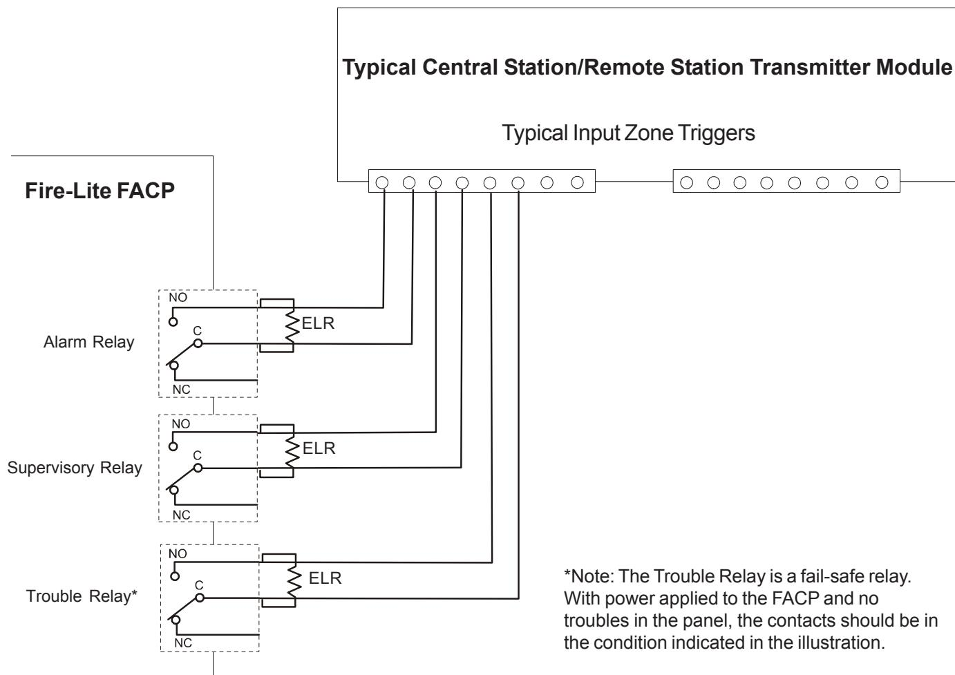
\*Note: The Trouble Relay is a fail-safe relay. With power applied to the FACP and no troubles in the panel, the contacts should be in the condition indicated in the illustration.
