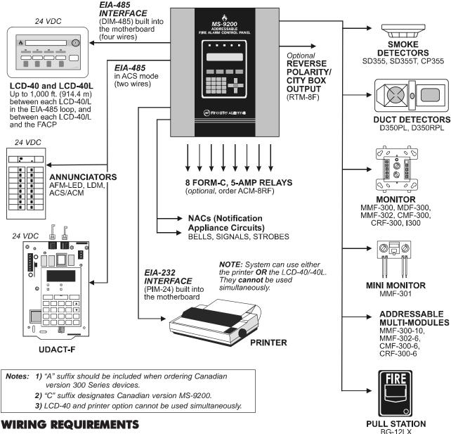
The SLC requires use of a specific wire type to ensure proper circuit operation. It is recommended that all SLC wiring be twisted-pair shielded to minimize the effects of electrical interference. Wire size should be no smaller than 18 AWG (0.78 mm²) and no larger than 12 AWG (3.1 mm²) wire.
