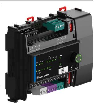
The Actuator Control Module has an optional Fail-Safe Module (FSM) that allows the valve to be moved to a preprogrammed position (Full Open, Full Closed, or anywhere in between) in the event of a power failure to keep the critical environment safe for the occupants and vital material inside. The Fail-Safe Module can be ordered as an option on valves or as an add-on later and has a simple plug-and-play connection.
