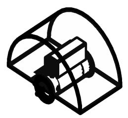
Supply valves will come standard with insulation while exhaust valves will come standard without insulation.
