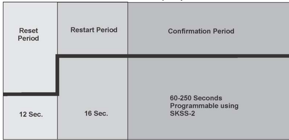
Figure 10-9 Smoke Verification Cycle
