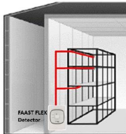
Figure 3: Example of in-rack air sampling
