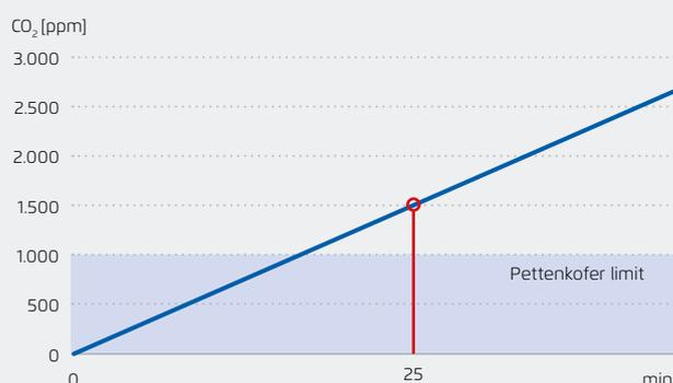
Without a fresh air supply, a CO<sub>2</sub> level of 1,500 ppm is reached in a classroom of 30 schoolchildren after just 25 minutes. The Pettenkofer limit for «good air» (hygienically harmless) stands at 1,000 ppm. Ventilation behaviour should be checked and, if the level is 1,000 ppm or more, action should be taken to improve it.
