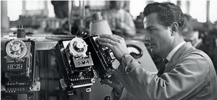
Time switches for automatic staircase lighting systems
