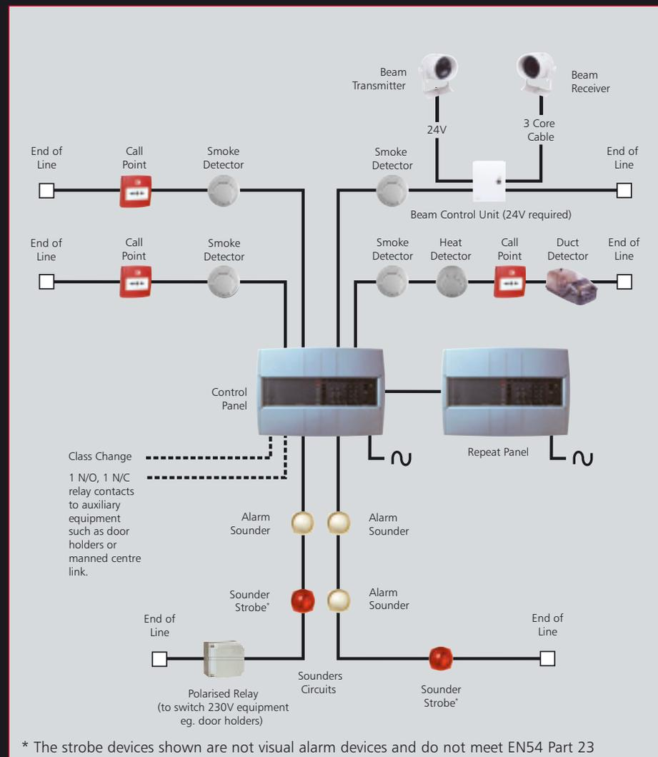
\* The strobe devices shown are not visual alarm devices and do not meet EN54 Part 23
