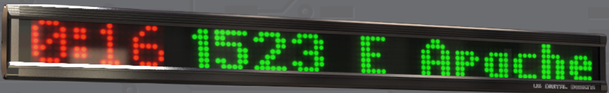
Extended Message Sign show a turnout timer along with alerted units and incident information.
