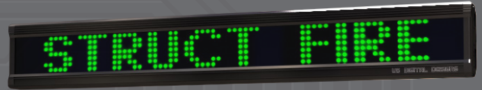
Standard Message Sign shows incident information and a turnout timer or unit number.
