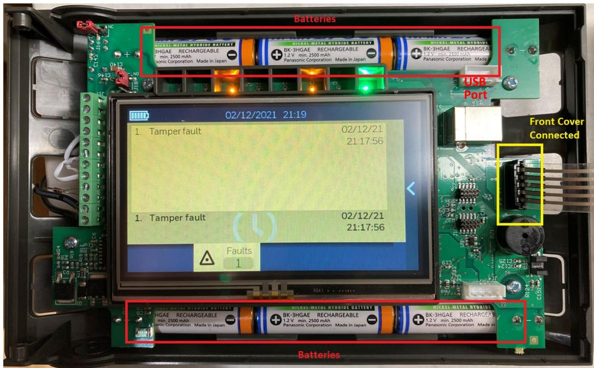
4. Connect a USB cable from a PC to the USB port on the Panel, as indicated above.
