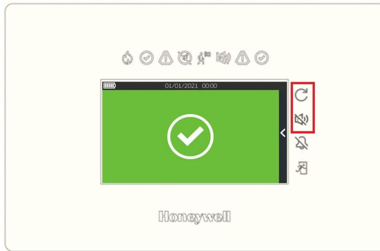
Keep the buttons pressed for approximately 5 seconds, until the Panel enters the **Bootloader Mode**. Once in Bootloader Mode (characterised by a continuous buzzer sound and blank display), release the buttons.
